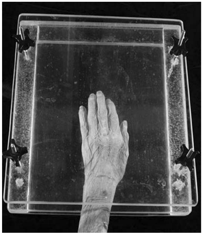
FIG. 1—The "Hand Press". This is the device that was used to position the cadaver hands for the posterior-anterior hand X-rays.
